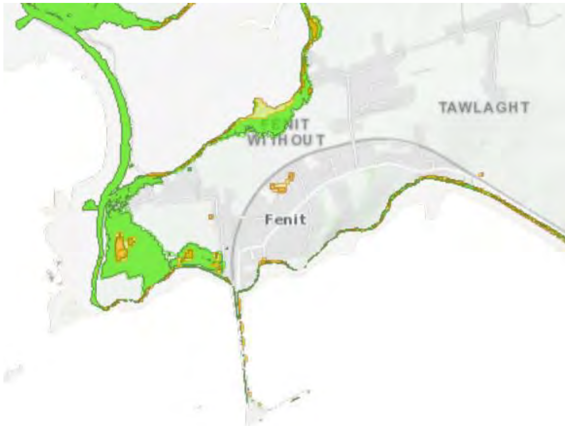
Figure 5-1 Flood Extent Mapping (ref: OPW)
